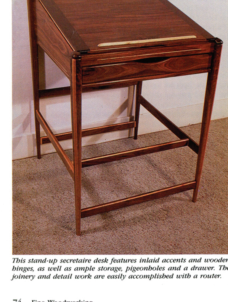
This stand-up secretary desk features inlaid accents and wooden hinges, as well as ample storage, pigeonholes and a drawer. The joinery and detail work are easily accomplished with a router.
