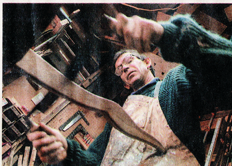
Prowell uses a draw knife to shape part of a standing mirror in his Sebastopol shop.
