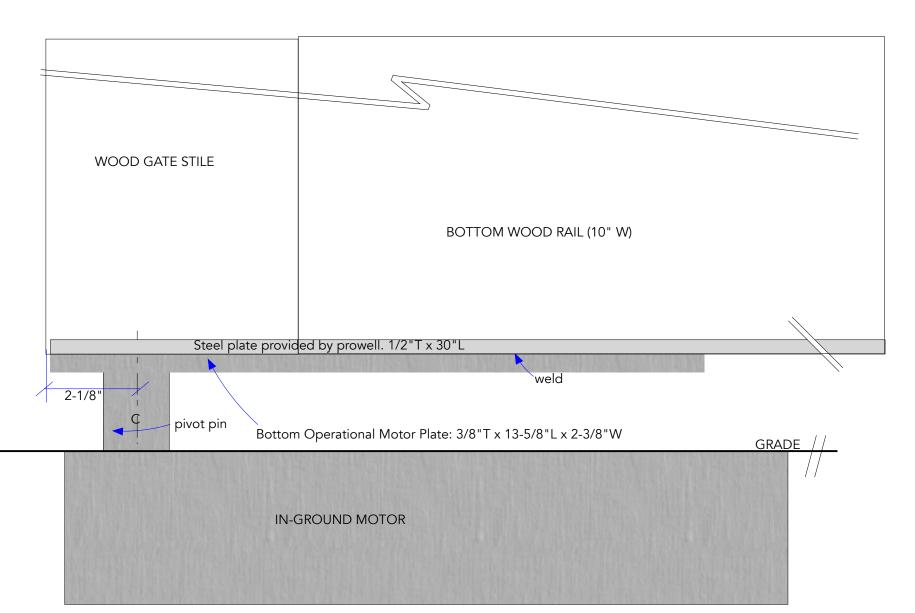
SIDE ELEVATION Left Gate Hinge edge
