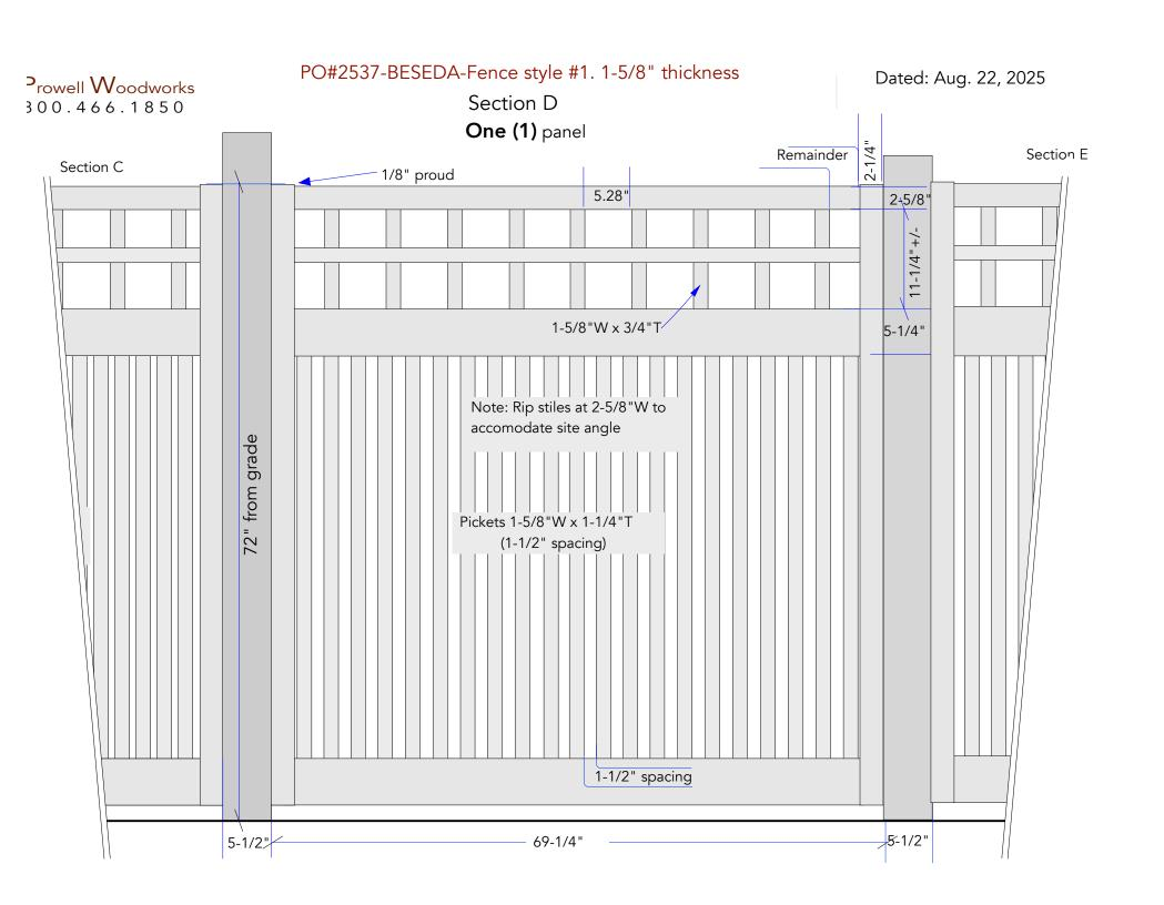
Prowell Woodworks PO#2537-BESEDA-Fence style #1. 1-5/8" thickness Dated: Aug. 22, 2025 800.466.1850 Section E One (1) panel 2-1/4" Section D Remainder 1/8" proud 5.28" 2+5/8" 11-1/4"+/-5-1/4" Pickets 1-5/8"W x 1-1/4"T (1-1/2" spacing) 1-1/2" spacing
