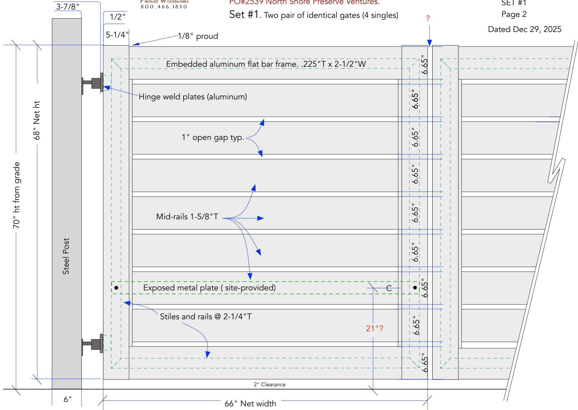
NOTES: Motor arm is at 18-1/2" from grade? Concrete motor footing is formed such that the motor arm mounts to the center of the 3rd rail from the bottom, at 21".(To be field verified)
